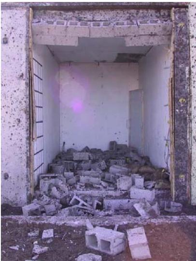
Figure 7. Post-Test view of control wall retrofitted wall
