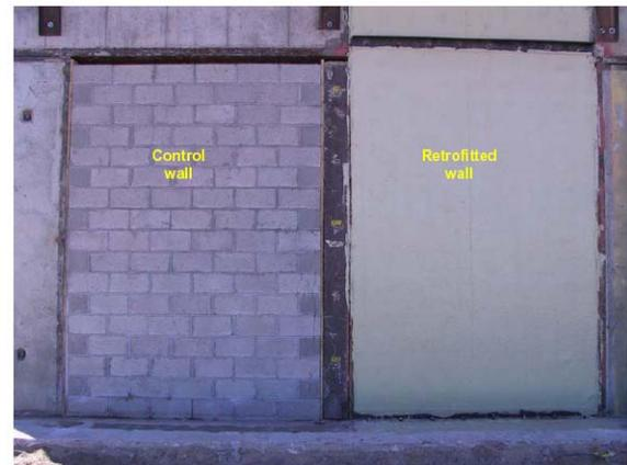
Figure 2. Containment Structure with Control and Retrofitted
